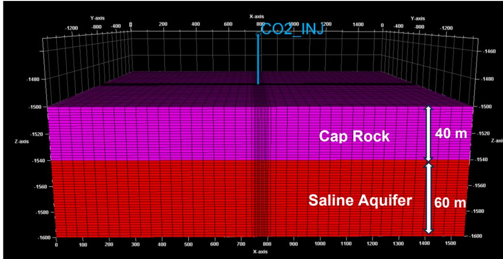
Figure 1: 3D Model representing the CO<sub>2</sub> injection in Saline Aquifer
