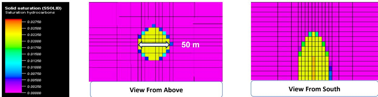
Figure 2. 3D Solid Saturation plot at 1.0 M-Ton/yr injection rate
