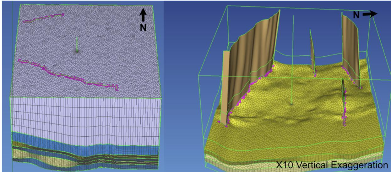
Figure 4. Saline field model mesh. Undifferentiated overburden sediments are shown in purple, mapped shale sealing units are shown in blue, mapped sand reservoir units are shown in yellow, and grid cells that are intersected by mapped faults are shown in pink. The full model is shown on the left and only the sandstone reservoirs and faults are shown on the right. The model is 7.8 km in length in the X direction, 8.2 km in the Y direction, and is between 1.8 km and 2.4 km in depth below mudline.
