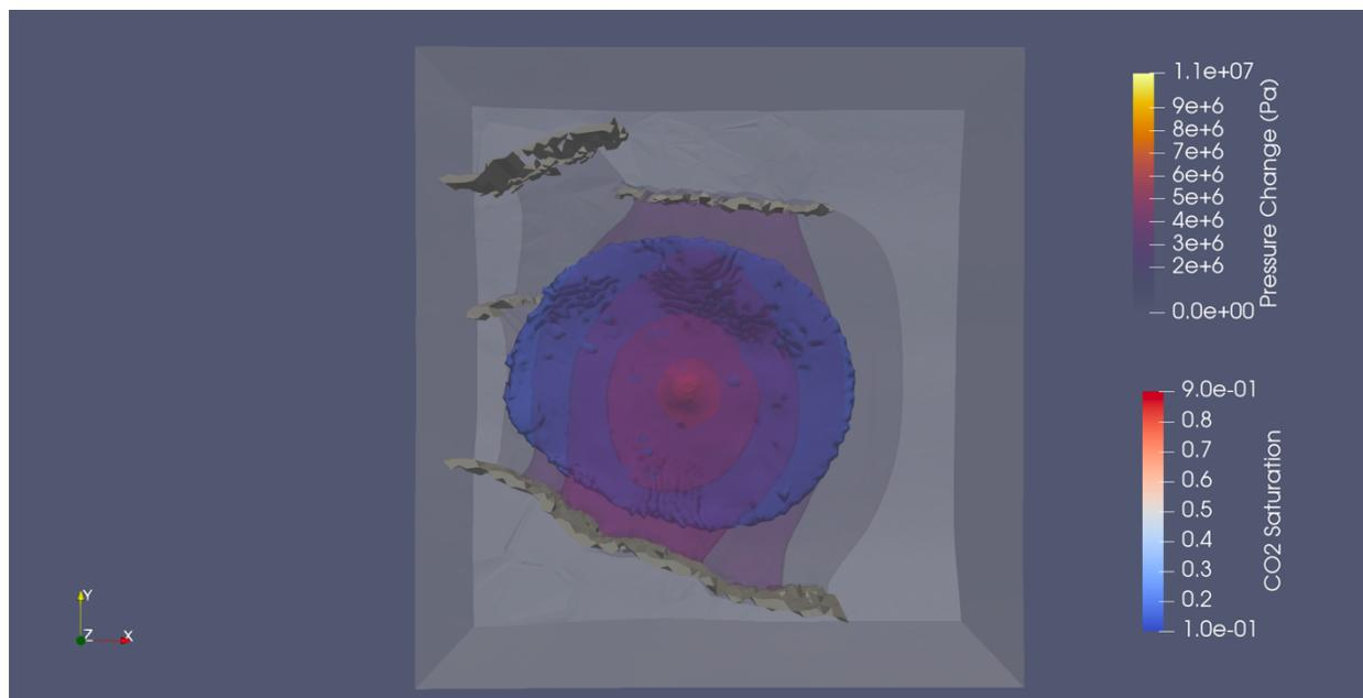
Figure 6. Saline field simulation results. The extent of the CO<sub>2</sub> plume is shown in blue with the extent of the related pressure plume shown on a scale from black to yellow. Faults are shown in gray. As the injection site sits at a local structural low point, injected CO<sub>2</sub> and pressure moved up-dip towards the North and South. The pressure front backs up against the faults, applying as much as 3.3 MPa of pressure increase, which poses risks for pressure-induced alteration.
