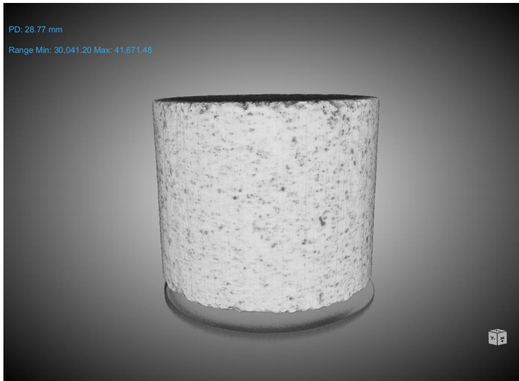
Figure 7a. Industrial CT scan image of dry Sample 3, showing the pore space in the limestone plug before exposure to \text{scCO}_2 .
