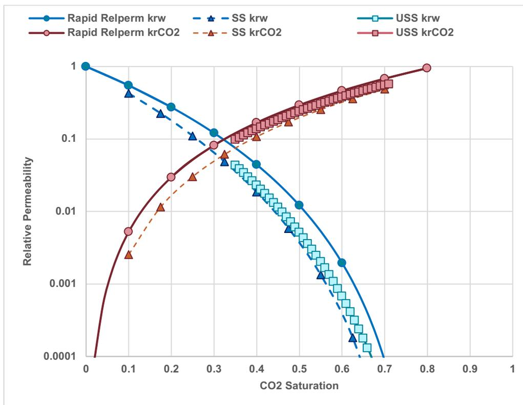
Figure 2: Final result is reservoir-condition relative perm curves that cover a wide range of expected fluid saturations. Diamonds are uncorrected steady state data and squares are uncorrected unsteady state data. Circles are capillary-pressure corrected USS relative perm. The simulation provides relative perm that is most representative of the true reservoir conditions.
