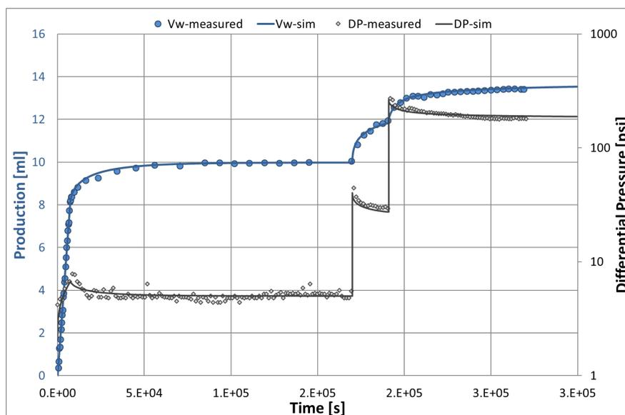
Figure 1. Circular dots show the cumulative brine displacement and diamond shapes show the differential pressure vs time.
