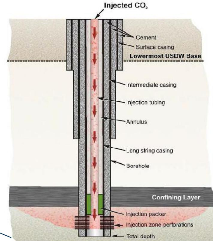
Schematic of injection well
