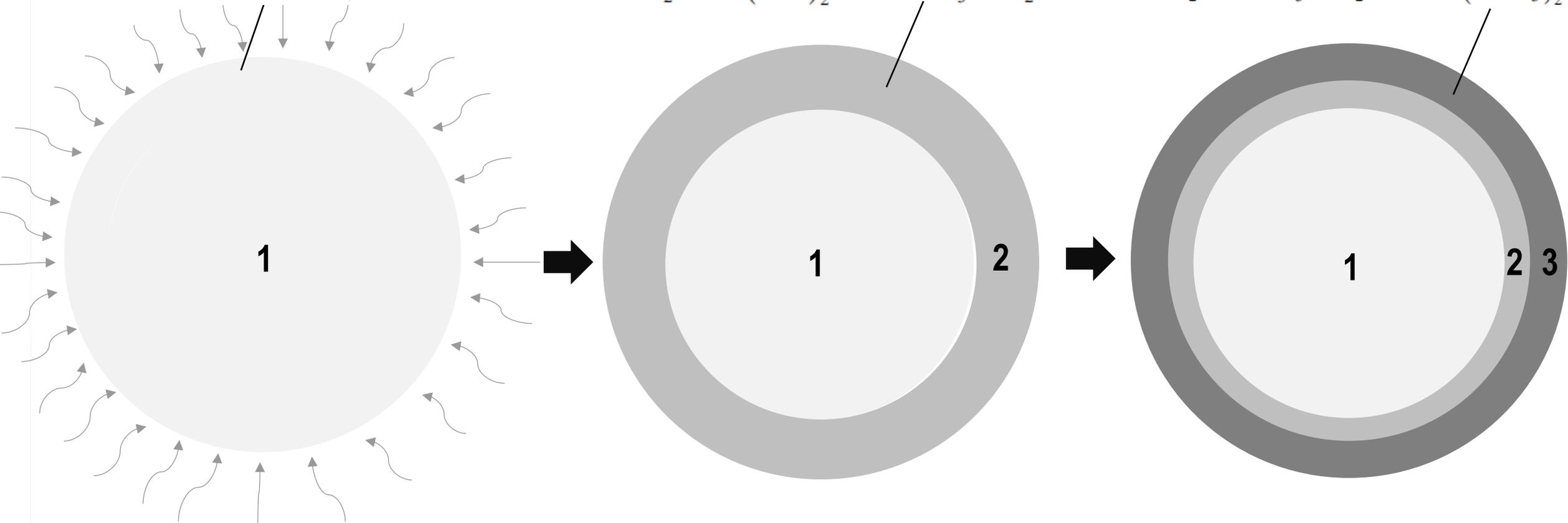
Plug is submerged in CO<sub>2</sub> saturated brine – CO<sub>2</sub> is diffusing into the cement through its circumference.
