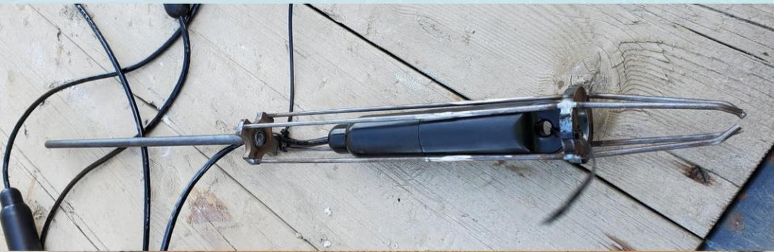
3 sensors per string; 2 strings taped together; bottom sensor installed in a metal cage to push sensor string down the hole.
